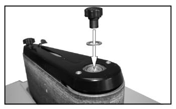
• Place the backstop into position and secure in place with the backstop securing bolt.
